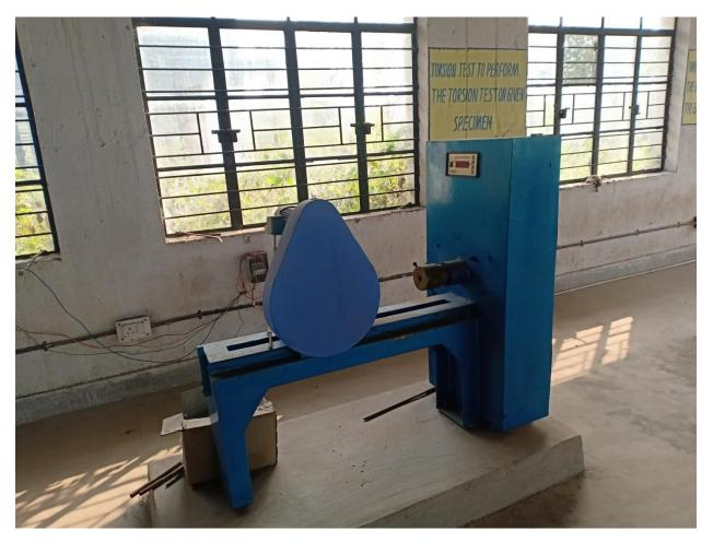
• Torsion test of mild steel rods has been done by the apparatus
