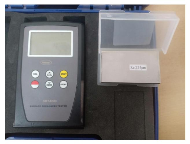
Measurement of surface roughness of given work piece
